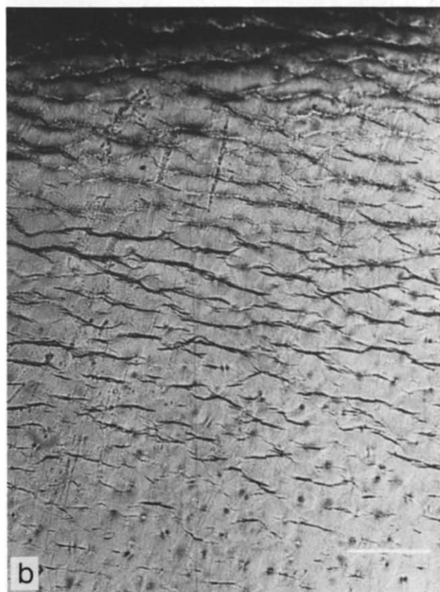
Figure 6 Trans-spherulitic and interspherulitic fissures in PVDF (a) \sim 1 mm below fracture surface; (b) immediately below fracture surface. Scale bar = 0.1 mm
